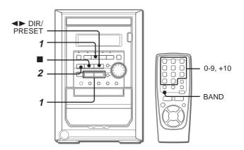
The unit can store a total of 32 preset stations (Each band has a maximum of 20 available preset stations). When a station is stored, a preset number is assigned to the station. Use the preset number to tune in to a preset station directly.
