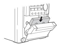
Insert a tape with the exposed side down. Push the cassette holder to close.
